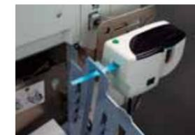
Notes: The Receiving Tray Paper Guide must be changed in the RISO Job Separator IV: NIII high-speed mode. The RISO Job Separator IV:NIII high-speed mode is not available with the RISO Auto-control stacking tray.
