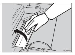
**I** If you could not remove the misfed master in steps **2** and **3**, take out the drum and remove the misfed master from the inside.
