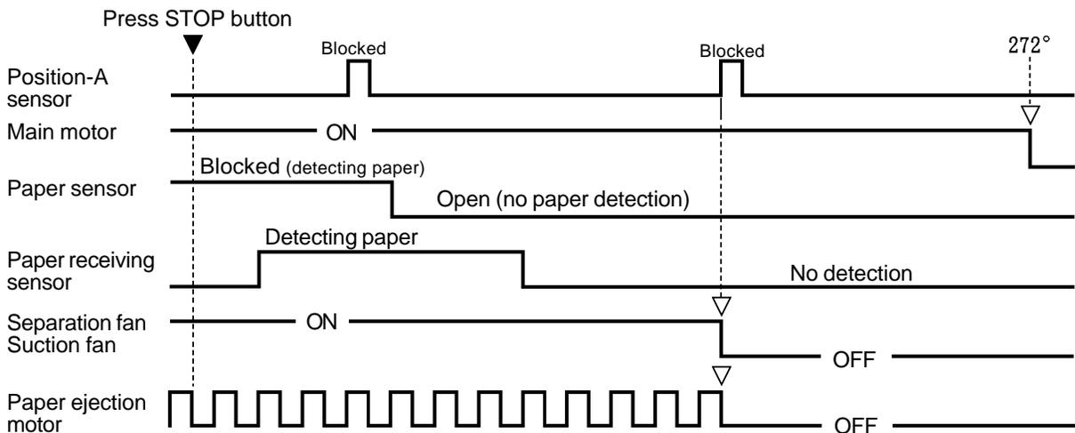
Note: If overload current is detected for **0.3 seconds** on the Paper ejection motor, Paper ejection motor lock message [E 20] is indicated.
