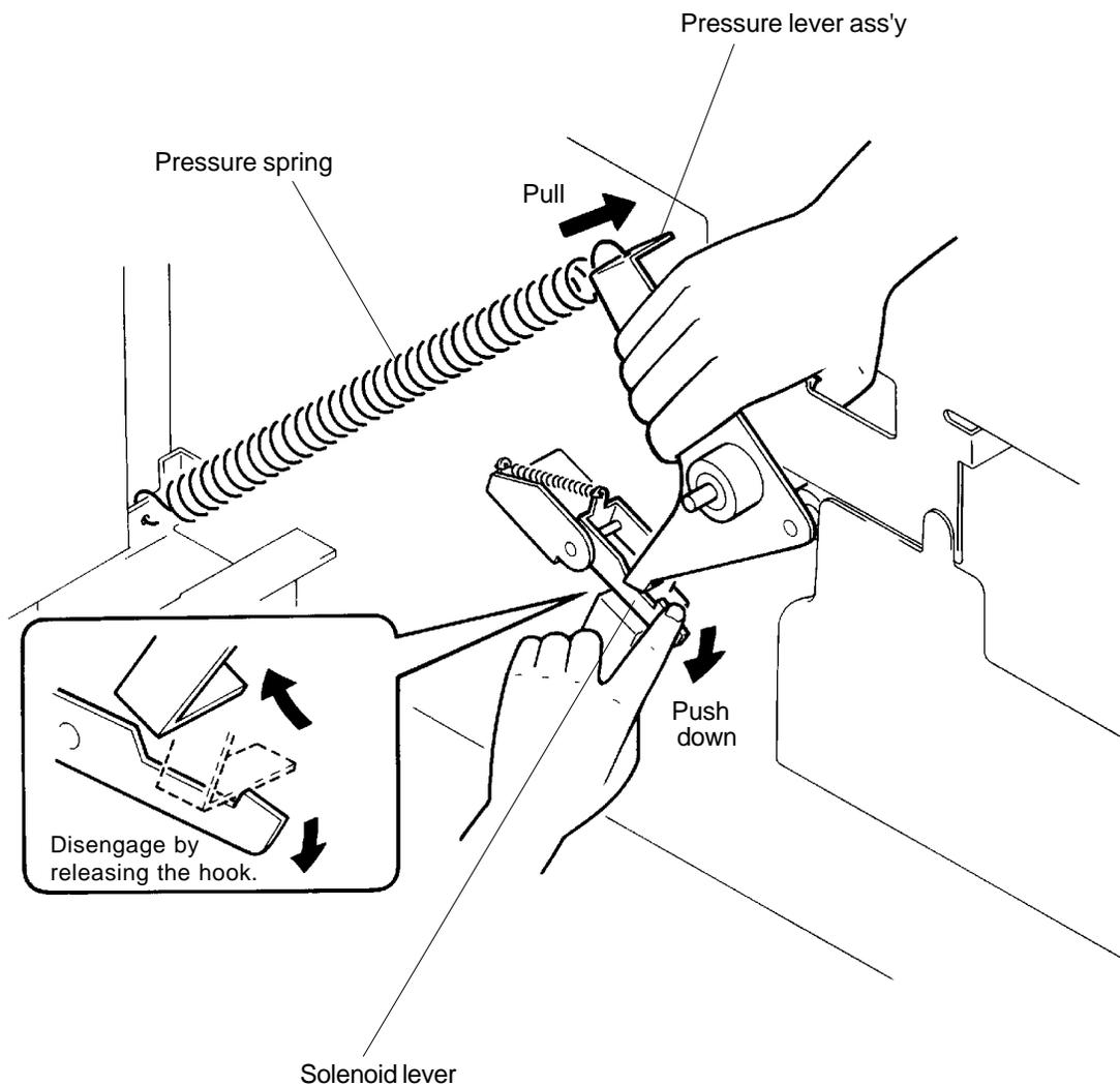
6. Carefully, remove the Pressure spring.
