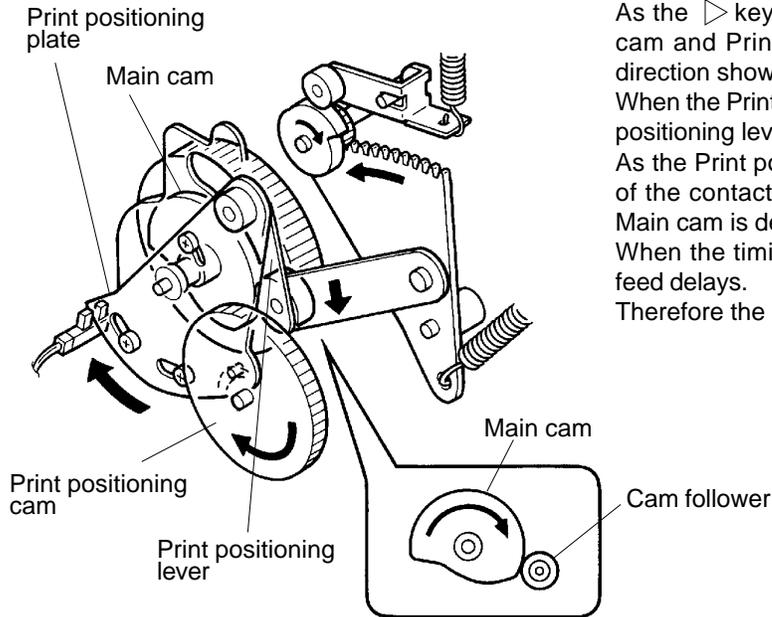
As the ▷ key is pressed, the Print positioning cam and Print positioning plate moves in the direction shown by the arrow marks.
