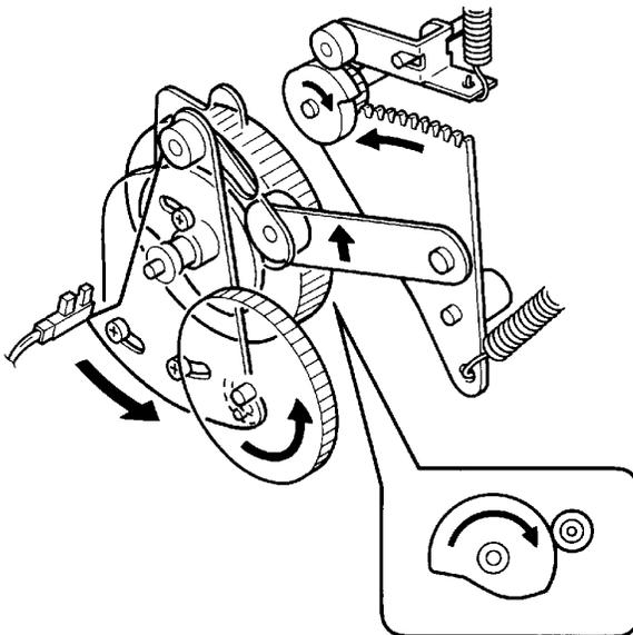
As the ◁ key is pressed, the Print positioning cam and Print positioning plate moves in the direction shown by the arrow marks.
