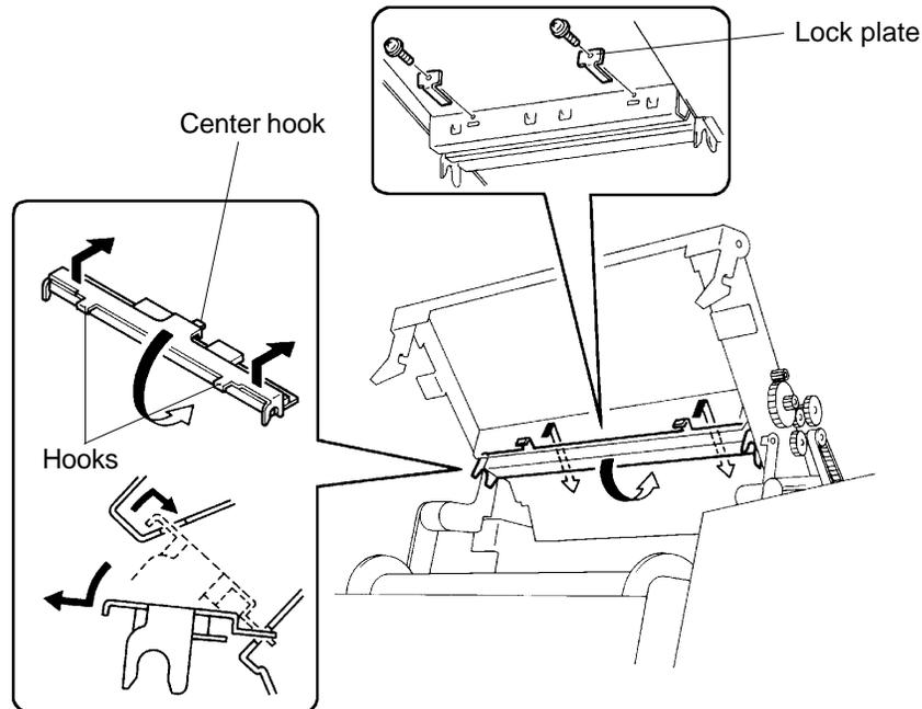
6. Disconnect two Connectors and one ground wire from the TPH, and remove the TPH.
