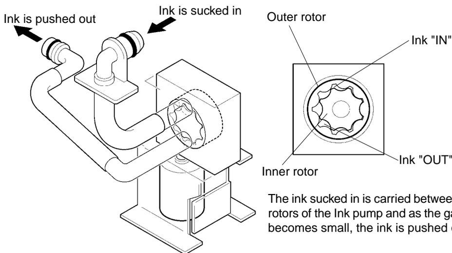
The ink sucked in is carried between the Outer and Inner rotors of the Ink pump and as the gap between the rotors becomes small, the ink is pushed out.
