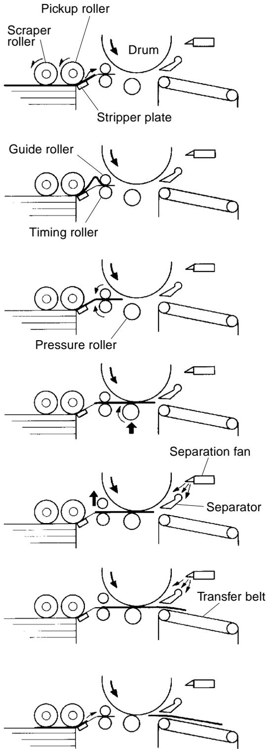
The Drum is rotated and a sheet of paper is fed from the first paper feed area to the second paper feed area by the Scraper and Pickup rollers, and Stripper plate.
