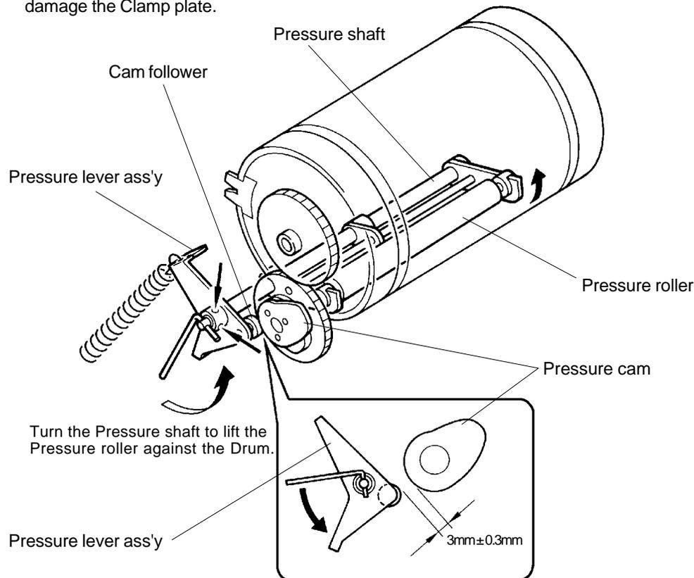
Turn the Pressure shaft to lift the Pressure roller against the Drum.
