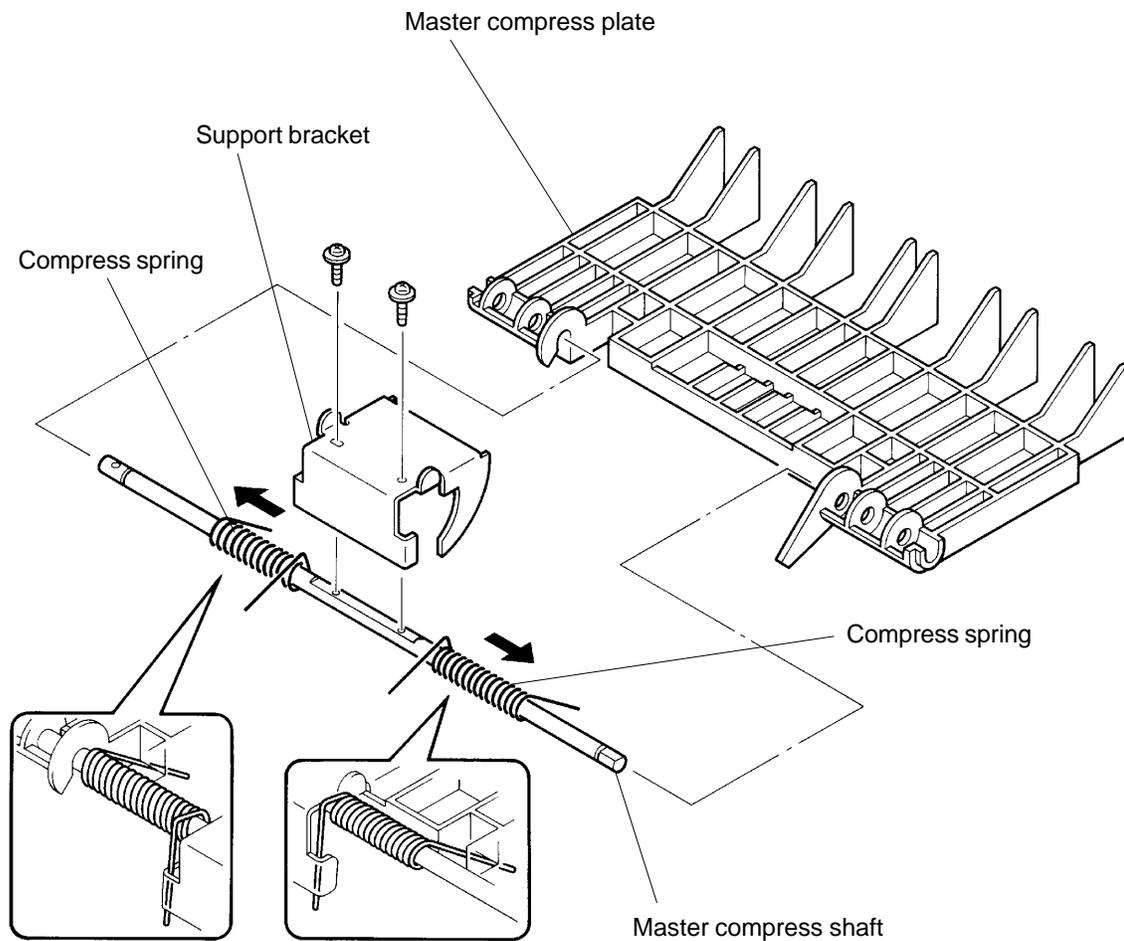
Hook the Compress springs in the correct direction and position.
