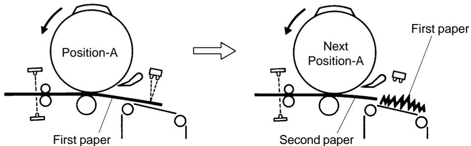
Paper does not escape from Paper receiving sensor from one Drum position-A to the next.
