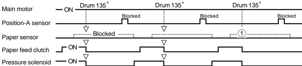
① The Paper sensor does not detect any paper within the third Drum rotation and displays [C 33].
