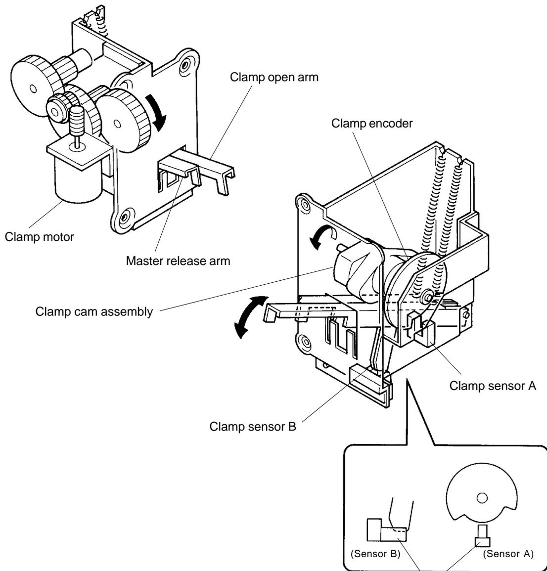
The light paths of the Clamp sensors A and B are both opened at Home position.
