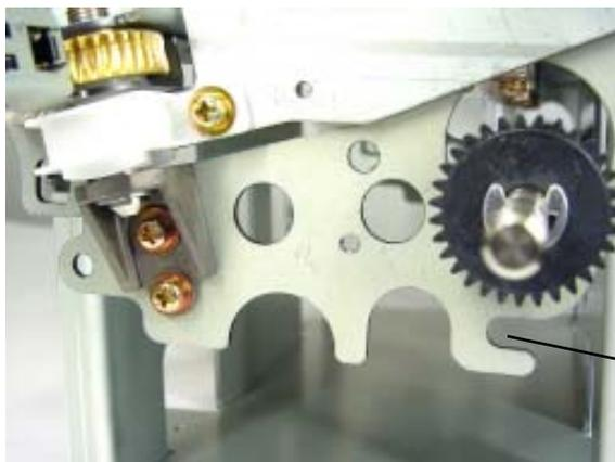
Slot in the Inner pressure roller support plate.
