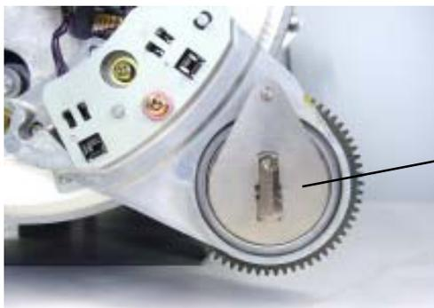
Drum joint alignment lock (JIG)
