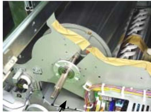
Insert a hand through this opening to support the paper drum.
