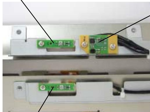
Multiple paper feed detection sensor (receive)
