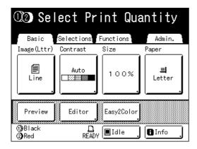
Input the number of copies prior to creating the master, because when "Auto-Process" is set, the job will be printed as soon as the master is created on Cylinder (Drum) 1 or Cylinder (Drum) 2.
