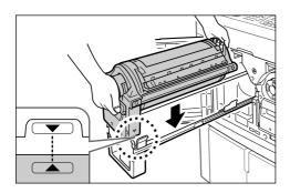
Align the ▼ mark on the Print Cylinder (Drum) with the **\( \Lambda \)** mark on the guide, and place the Print Cylinder (Drum) horizontally onto the guide.
