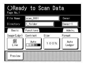
The data name, save location and owner name are automatically allocated when scan mode is started, but you can change this preset information if needed.
