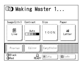
Once the masters are made, one proof copy from Cylinder (Drum) 1 alone is printed, and the Master Making Basic Screen for Cylinder (Drum) 2 appears.
