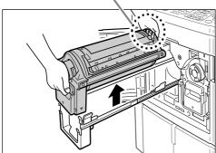
Use both hands to lift the Print Cylinder (Drum) straight up to remove from the rail. Proceed with replacing the cylinder (drum), removing the paper jam, etc..
