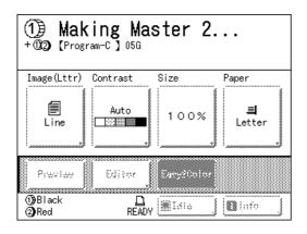
Once the master is made on Cylinder (Drum) 2, a single 2-color proof copy will be printed. After a proof copy has been printed, the Print Basic Screen appears.
