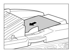
Use the ADF unit if you are printing multiple originals in succession. Place originals facedown and then adjust the ADF Original Guides to the width of the originals. Insert the originals as far into the ADF unit as possible.
