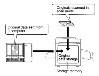
Stored data is managed as "Storage Data", and unless expressly deleted, will not be cleared if you press the (REBET) key or turn the machine off.
