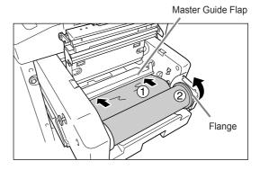
Insert the leading edge of the master into its entrance under the Master Guide Flap and advance it as far in as it will go ( 1). If the Master is loose, turn the flange at the right towards the rear and rewind (2).
