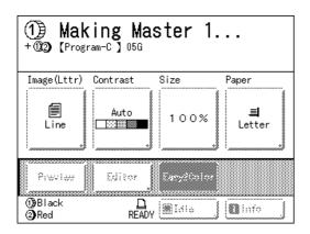
Once the master is made on Cylinder (Drum) 1, one proof copy will be printed from Cylinder (Drum) 1 only. A master will then be made on Cylinder (Drum) 2.
