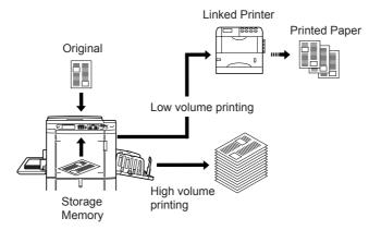
Automatically select an output device based on number of copies when printing from a computer. (When "Online Auto-Link" is enabled) ☞p.165
