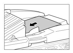
The ADF unit detects the document, and automatically opens the Master Making Basic Screen
