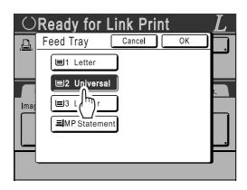
2) Touch the button corresponding to the size of the paper loaded in the "Universal" tray.
