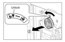
Turn the Ink Cartridge to the counter clockwise ('t) and then pull it out.
