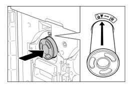
Align the arrow on the Ink Cartridge to the \(\bigvarboldsymbol{\psi}\) mark on the cylinder (drum) unit, and insert until it stops.
