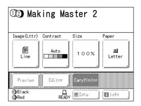
Once the master is made on Cylinder (Drum) 2, a single 2-color proof copy will print from Cylinder (Drum) 2.
