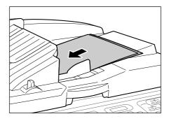
If you are using the ADF unit, you can set the original and the Area Specification Sheet at the same time. If you do so, place the sheet on top of the original.
