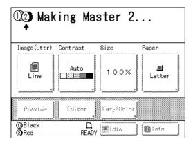
Once the master is made, a proof copy using only Cylinder (Drum) 2 is printed, and then a 2-Color proof copy is printed.
