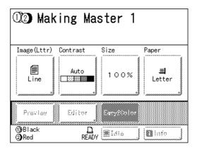
Once the master is made on Cylinder (Drum) 1, one proof copy will print from Cylinder (Drum) 1 only. A master will then be made on Cylinder (Drum) 2.
