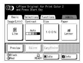
In step 5, if two originals have been placed together in the ADF unit, one proof copy from Cylinder (Drum) 1 only is printed, and the master is subsequently made on Cylinder (Drum) 2. Continue on to step 11.
