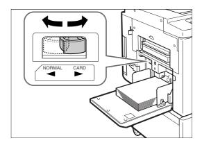
Position the Paper Feed Pressure Adjustment Lever according to the finish of the paper. NORMAL: For standard paper CARD: For thick or smooth-surface paper
