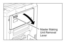
Grasp the Master Making Unit Removal Lever and pull out to open.
