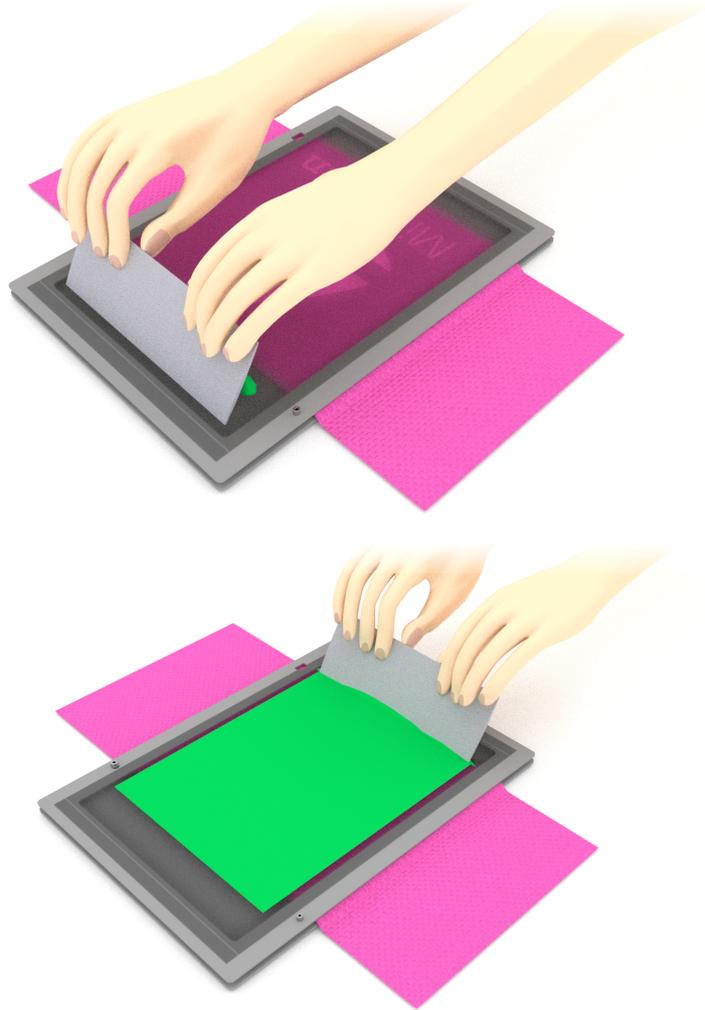
Replacing the substrate after each print enables consecutive printing.
