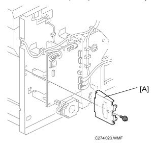
1. Remove the bracket [A] (Fx1).
