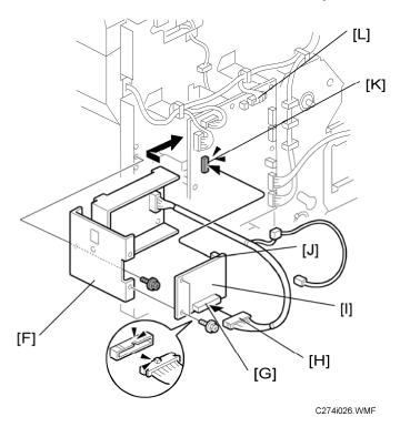
4. Attach the bracket assembly [F] to the same place that the bracket [A] (Step 1) was installed (1 screw).
