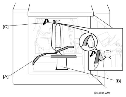
3. Remove the front tape [A], the tag [B], and the rear tape [C].
