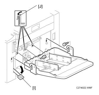
14. Lower the paper feed tray adjustment lever [I], and install the paper table.( F x 2)
