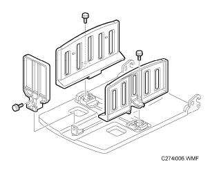
15. Attach the side and end fences, as shown. ( F x 3)
