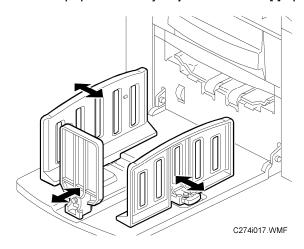
20. Adjust the side and end fences of the paper delivery table to match the paper size.
